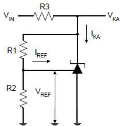
Figure 5. Test Circuit 5 for  $V_{KA} = V_{REF} \cdot (1 + R_1/R_2) + I_{REF} \cdot R_1$
