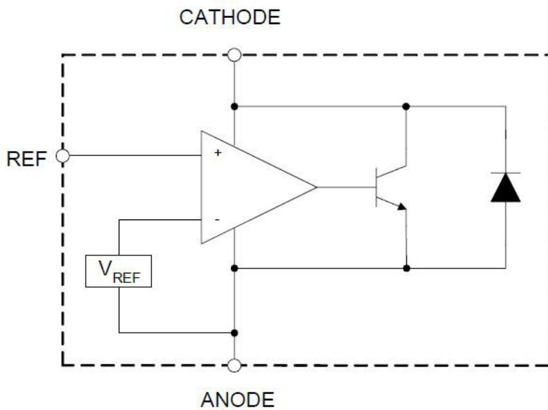
Figure 3. Functional Block Diagram of FL431A
