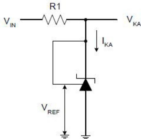
Figure 4. Test Circuit 4 for  $V_{KA} = V_{REF}$
