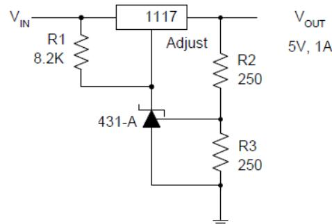
Figure 10. Precision 5V 1A Regulator
