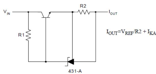
Figure 9. Current Source or Current Limit
