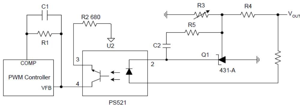
Figure 11. PWM Converter with Reference
