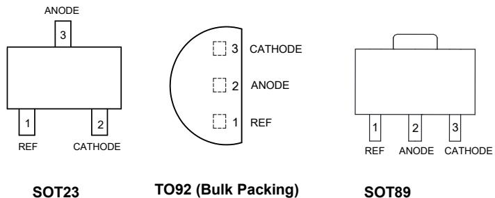
Figure 2. Pin Configuration of FL431-A(Top View)
