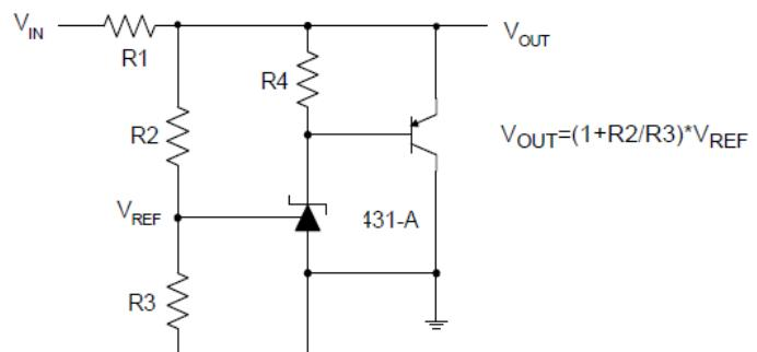
Figure 8. High Current Shunt Regulator
